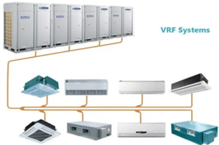
Figure 2: VRF air conditioning system
