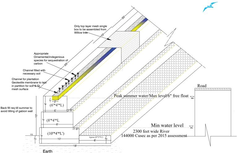
Note: 4" joint to be provided for next gabion wall in req allignment.
