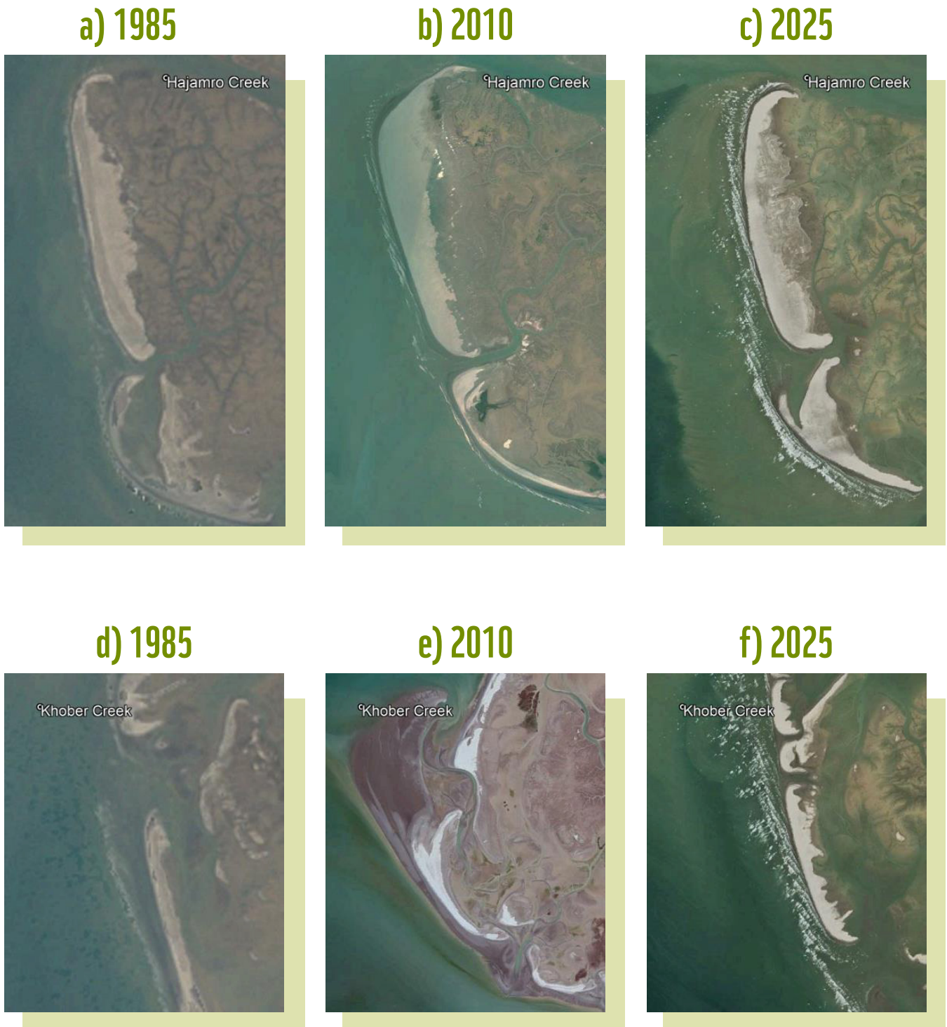
Figure 2: Shoreline change over different years, as witnessed by Google Earth Images Hajamro (a, b, c) and Khober Creek (d, e, f)
