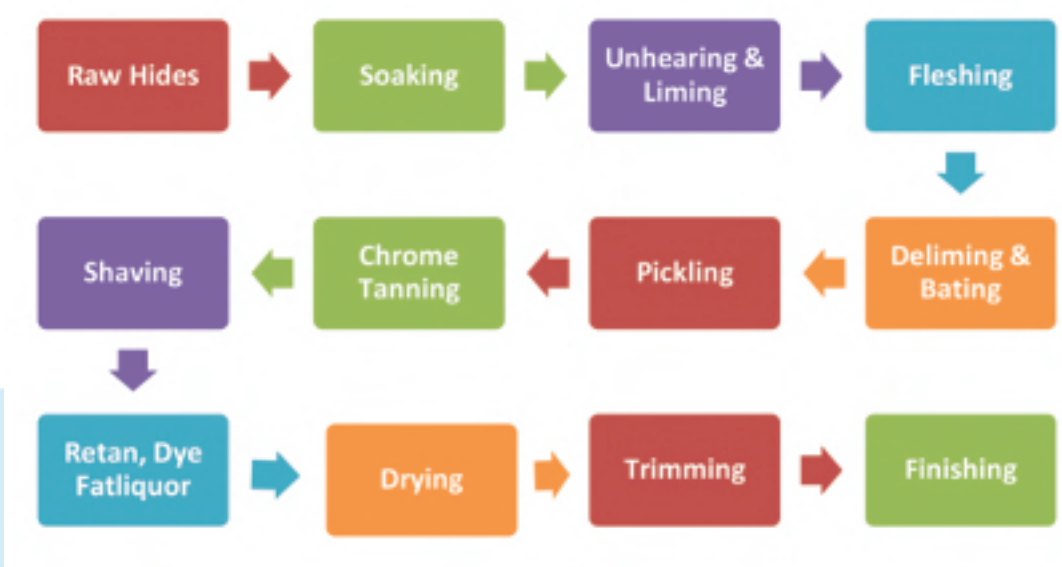
Figure 4-Process Flow Diagram of Leather Production
